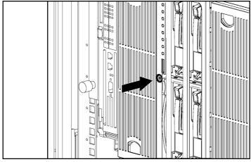
Figure 1-1: Pressing the Power On/Standby button
